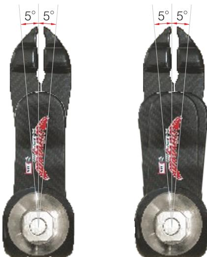
Thanks to its split lines on main plate, pyramid section of the foot easily rotates around center of the pyramid and causes +/- 5 degrees of torsion.
